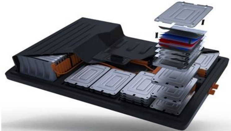
EV car battery pack
